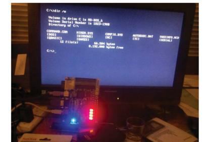
FPGA configured to behave like an Intel 8086 microprocessor demonstrating MS-DOS 6.22
